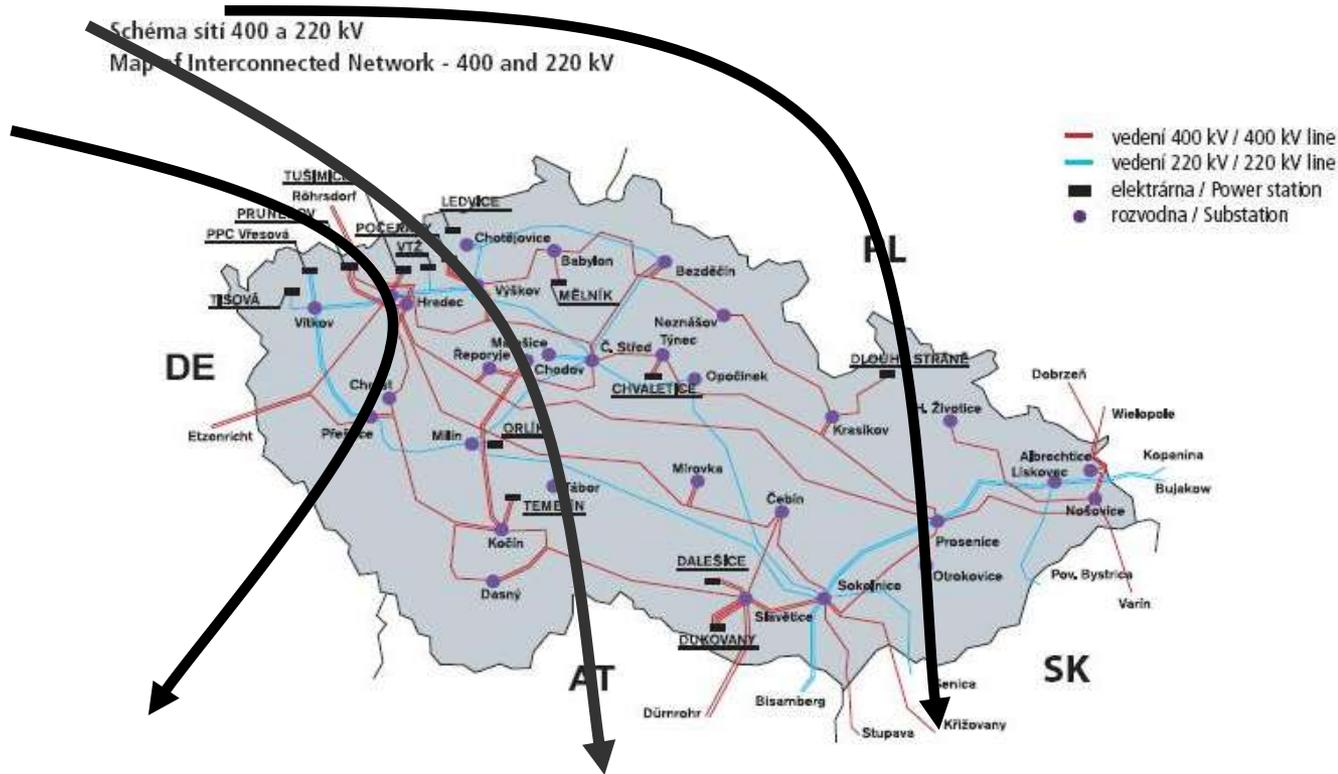
Problem: Loop flows from N. Germany to S. Germany and Austria, end of 2014: > 3400 MW from Germany to Austria
